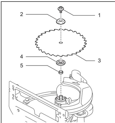
► 1. Hex bolt 2. Outer flange 3. Circular saw blade
