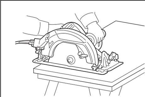
Hold the tool firmly. The tool is provided with both a front grip and rear handle. Use both to best grasp the tool. If both hands are holding saw, they cannot be cut by the circular saw blade. Set the base on the workpiece to be cut without the circular saw blade making any contact. Then turn the tool on and wait until the circular saw blade attains full speed. Now simply move the tool forward over the workpiece surface, keeping it flat and advancing smoothly until the sawing is completed.
