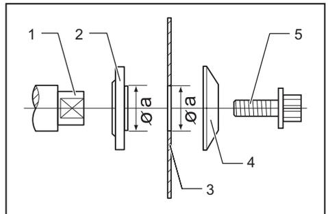
► 1. Mounting shaft 2. Inner flange 3. Circular saw blade
